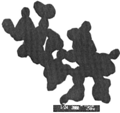
Fig. 2. Transmission electron micrographs for \text{LiMn}_2\text{O}_4 particles synthesized and calcined at 800^\circ\text{C} .
